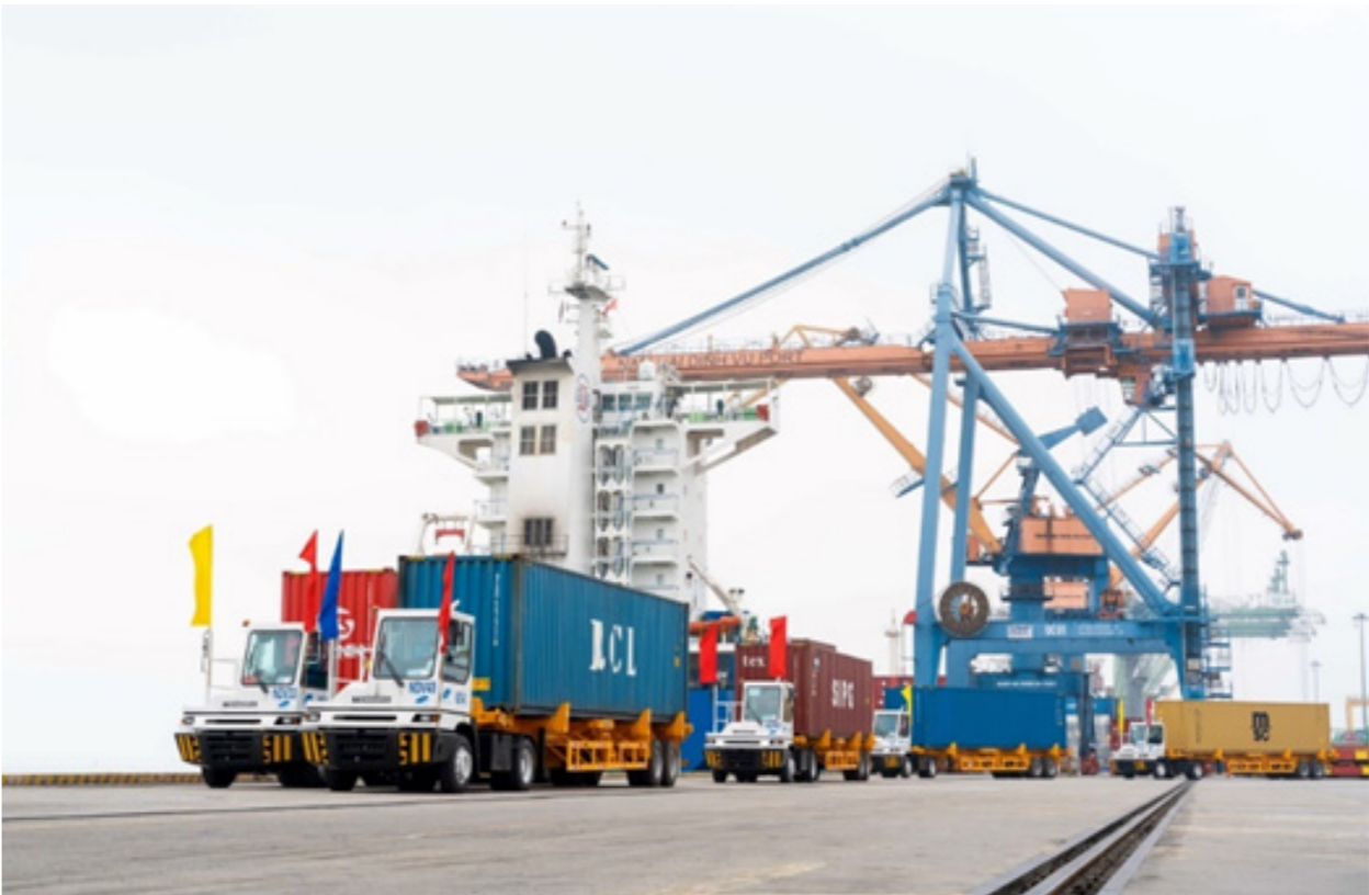
100% electric STS shore crane is being installed at Phase 2 of Nam Dinh Vu port
